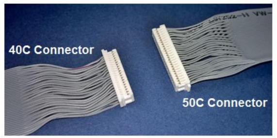
Ribbon Wire Flying Lead Part Number (40C) : QD6020 (Used with QD5747AD) Ribbon Wire Flying Lead Part Number (50C) : QD6022 (Used with QD5745AD)
