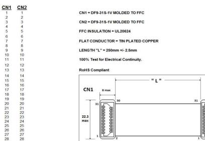
FFC DIMENSIONS: PITCH = 0.5 mm CONDUCTOR WIDTH = 0.30mm CONDUCTOR THICKNESS = 0.035mm TOTAL PITCH = 15 mm WIDTH = 16 mm MARGIN = +/- 0.15
