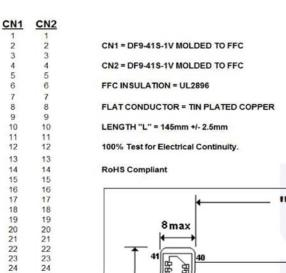
FFC DIMENSIONS: PITCH = 0.5 mm CONDUCTOR WIDTH = 0.30mm CONDUCTOR THICKNESS = 0.035mm TOTAL PITCH = 20 mm MARGIN = +/- 0.15
